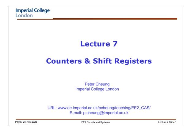
In this lecture, we will focus on two very important digital building blocks: **counters** which can either count events or keep time information, and shift **registers**, which is most useful in conversion between serial and parallel data formats. We will also learn about a special type shift register known as Linear Feedback Shift Registers, which are widely used to generate random digital numbers.
